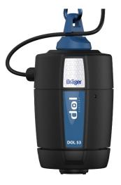
DOL 53 consists of an electro chemical diffusion sensor and signal processing electronics. DOL 53 works like a "nose". DOL 53 only transmits the concentration measured at the sensor. The measuring unit ppm (parts per million) is a volume concentration. DOL 53 is connected to suitable control unit over a 3-wire cable. The measuring signal during normal operation is between 0 V and 10 V
